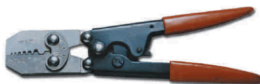
HEXPRESS F - 6 (for End Sealing Ferrules) Crimping Capacity : 0.5mm 2 to 6mm 2
